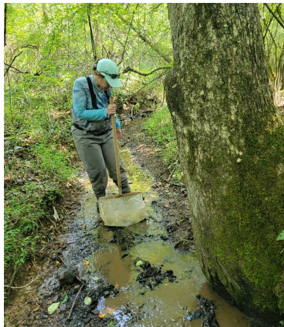
Figure 3.31. Sampling for benthic macroinvertebrates with TDEC protocols
